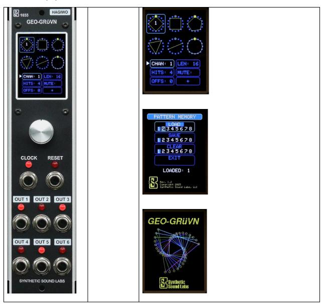
6 Channel Euclidean rhythm gate sequencer for Synthesizers.com format modular synths.
