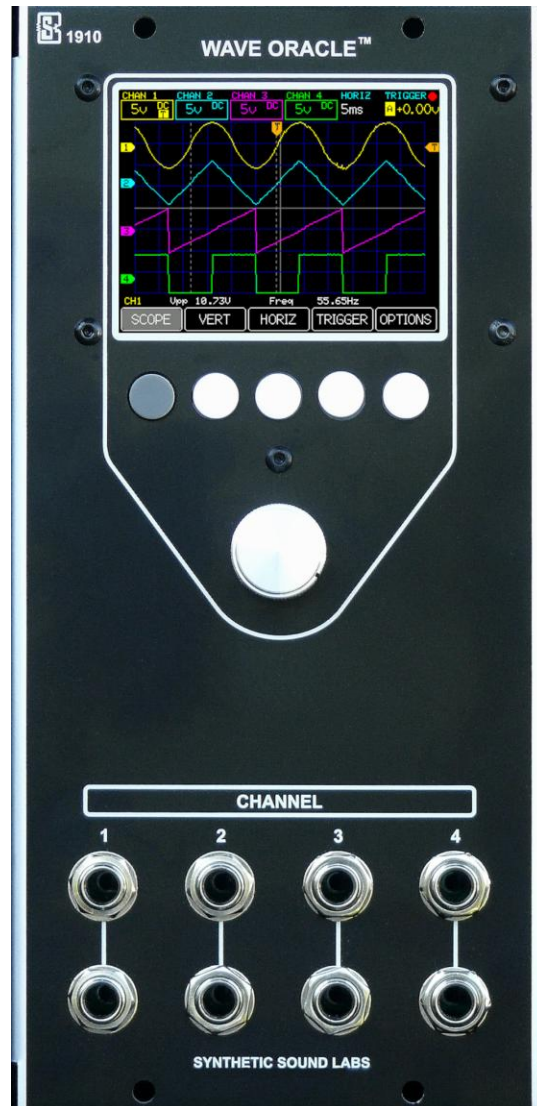
Five physical buttons below the display, a push encoder and four paired inputs.
