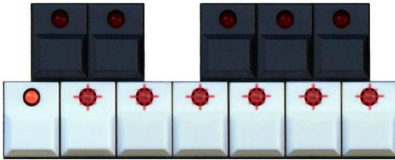
To select a different sequence, press the white note key corresponding to the sequence you want to select. If the sequencer is running, the newly selected sequence LED will flash until the sequencer reaches the end of the current sequence (or on the next clock; see CHANGE ON CLOCK mode), and will then switch to the new sequence.
